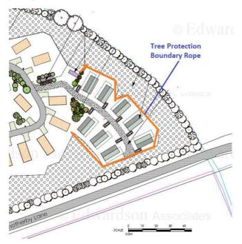
Boundary rope to be 10mm in size with hazard tape wrapped round.
